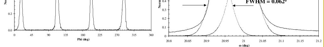
Φ scans CFO-PZT bilayer thin film<br/>deposited on MgO [1 0 0] substrate.<br/>The Bragg plane chosen for<br/>refection is [101] plane as it give the<br/>highest peak in powder.Rocking curve ( $\varpi$ -scan) of CFO(400)-<br/>PZT(200) peak showing a large<br/>degree of planar orientation<br/>[FWHM of CFO(400) peak is 0.062°<br/>at  $\Theta = 20.93°$  and<br/>FWHM of PZT(200) peak is 0.072°
