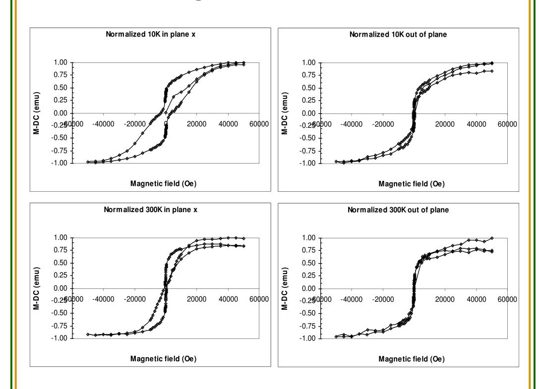
M vs H hysteresis loops of CFO-PZT (200nm-200nm) epitaxial bilayer on MgO substrate using PPMS measurements
